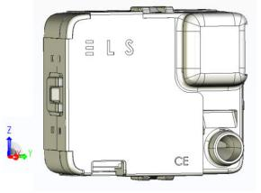
You can set the NextPS sensor in another device thanks to the two holes in the back of the sensor. The holes are made to receive self turret screw M2.5 and are 5 mm deep.
